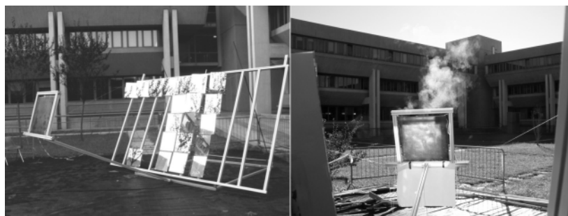
Fig. 11. – Left: mirror array of 20 elements with oven. Right: view of the oven with the water boiling (taken from behind the mirrors). The white paper fixed below the oven serves for reading the signal from the gauge mirror needed for regulating the system.
