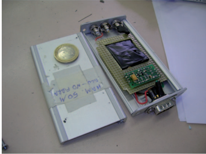
Fig. 4. – A counter assembly, showing the 3 by 3 cm 2 tile and the preamplifier.
