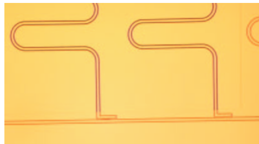
Fig. 12. – Microwave resonators coupled to a CPW line.
