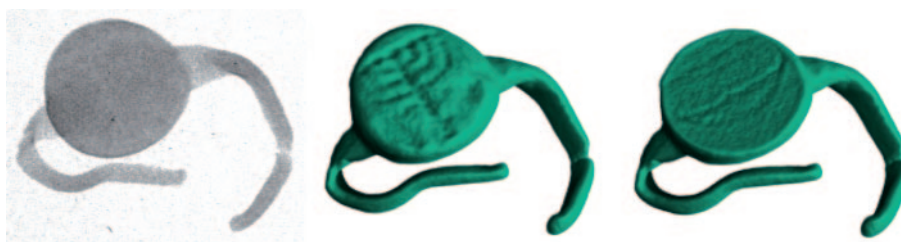
Fig. 3. – Neutron images of the same object, a Jewish finger ring with menorah sign from the Augusta Raurica settlement (Basel, CH): left—transmission image, middle—outer structure obtained by neutron tomography, right—virtual slice in the tomography data set near the boundary between the two parts of the ring.
