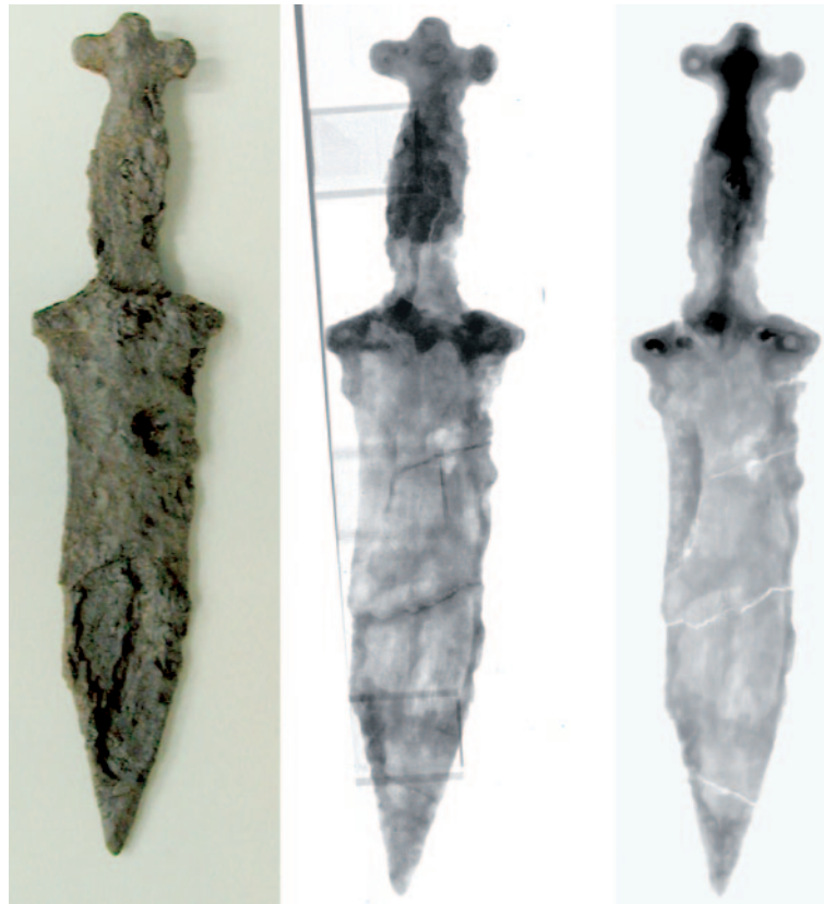
Fig. 5. – A dagger from excavations near the Roman Vindonissa camp (photo left) were inspected with neutrons (middle) and X-ray (right). Similar in first order, specific differences can be found out in respect to conservation measures and corrosion status.
