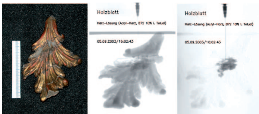
Fig. 8. – Inspection of the resin treatment of a wooden leaf where an injection takes place: left: photo of the object, middle: direct image of the arrangement, right: structure of the leaf withdrawn—the resin solution becomes directly visible.
