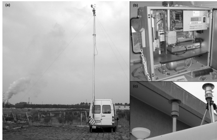
Fig. 1. – (a) Mobile laboratory with telescopic mast for meteorological measurements. (b) Sequential PM10 sampler Thermo ESM Andersen FQ95SEQ. (c) Particular of the sampling inlets (PM10 and PM2.5) and of the rain gauge.
