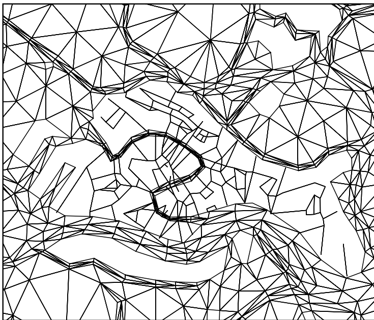
Fig. 5. – Coupling between the 2-dimensional model of the Venice Lagoon and the 1-dimensional model of the inner channels of Venice. It can be seen how the channel network fits nicely into the existing finite-element model grid of the Venice Lagoon.
