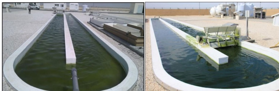
Fig. 1 Pictures of Picochlorum sp. (left) and Chlorocystis sp. (right) cultures in outdoor 25,000-L raceway ponds on 6th day of cultivation
