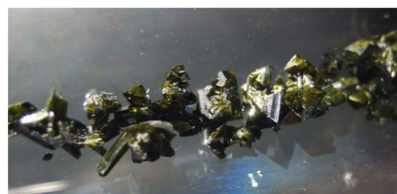
Fig. 1 Photography of crystals of UCl_4 , obtained by the described synthesis method. The height of the picture corresponds to \sim 15 mm.
