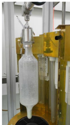
Figure S2. Fused quartz apparatus used for photoreduction.
