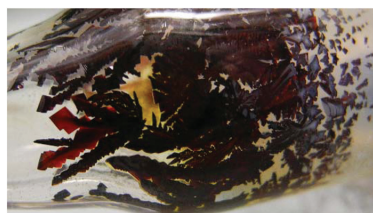
Fig. 3 Photography of \text{UBr}_4 -crystals inside the transport ampoule. The height of the picture corresponds to ~15 mm.
