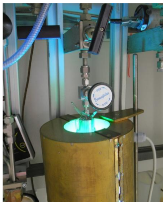
Figure S1. Photoreduction of UF 6 with CO in a UV-reactor.
