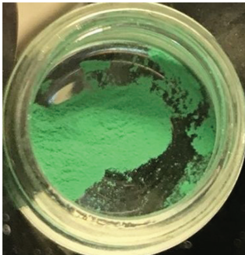
Fig. 2: UF_4 powder obtained from the reaction of UF_6 with S_8 in aHF.
