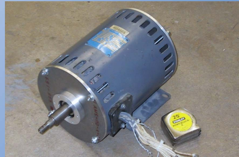
A 90 HP electric motor based on automotive duty.
