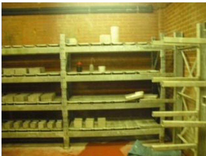
Figure 6. Keeping the temperature of test portion and water constant at 20°C in the curing room.
