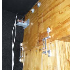
Figure 8. Monitoring knee rotations with “portal” strain gauges.
