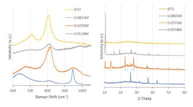
Figure 1. Raman spectra (left) and XRD patterns (right) of as-made BTO films and HTO films prepared from 0.0815, 0.0701, and 0.0538 M Na<sub>2</sub>WO<sub>4</sub> solutions, respectively. Legend orders match the spectrum/pattern orders top-to-bottom. The vertical lines under the 0.0701 M XRD pattern are from JCPDS card no. 35-1001 for hexagonal WO<sub>3</sub> · 1/3 H<sub>2</sub>O.
