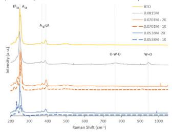
Figure 3. Raman spectra of selenized BTO films and HTO films prepared from 0.0815, 0.0701, and 0.0538 M  $Na_2WO_4$  solutions, respectively. Legend orders match the spectrum order top-to-bottom. 1X = one selenization cycle, 2X = two selenization cycles.
