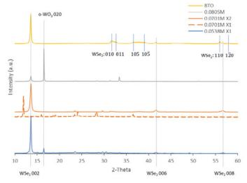
Figure 2. XRD patterns of selenized BTO films and HTO films prepared from 0.0815, 0.0701, and 0.0538 M  $Na_2WO_4$  solutions, respectively. Legend orders match the spectrum order top-to-bottom. 1X = one selenization cycle, 2X = two selenization cycles.
