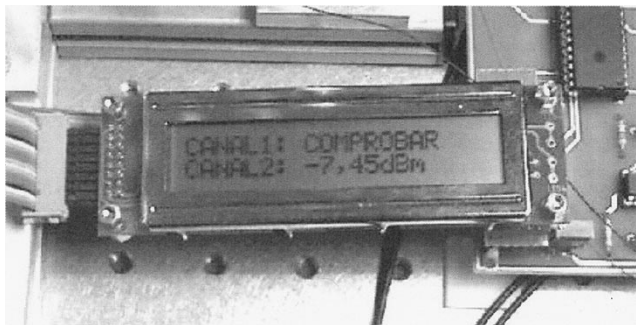
Fig. 4. LCD message showing output power at working channel (CH2) while CH1 must be revised (COMPROBAR).
