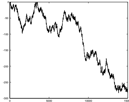
Figure 11. Realization of the process y_t = x_t - x_{t-1} ; where x_t is a random walk with Nid(0, 1) errors.
