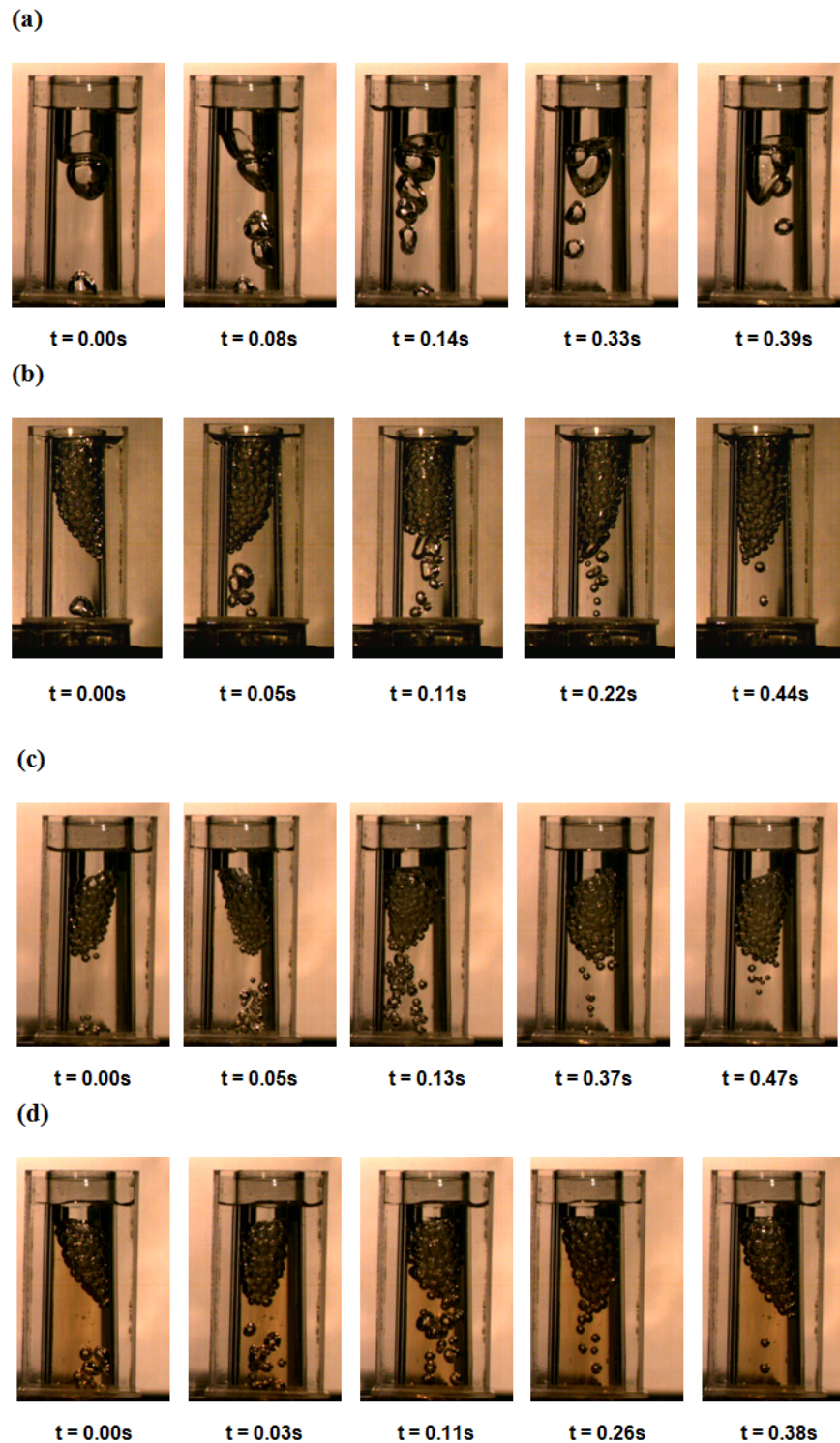
Figure 3.6. Visualisation of gas bubble number and size distribution in the REG plate design for (a) water (b) water with 0.5 \text{ g L}^{-1} Pluronic-F68, (c) CD-CHO media and (d) PPG. Experimental conditions: 7 mL fill volume; 650 rpm shaking frequency; d_o 2.5 mm; 5 \text{ mL min}^{-1} gas flow rate. Images taken as described in Section 2.2.6.
