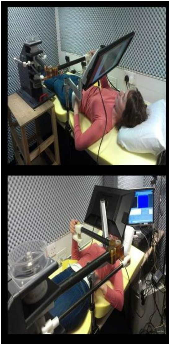
Figure 4.1: Participants were required to lie in the supine position whilst holding a robot manipulandum which controlled an on-screen cursor. Eye position and fixation was monitored in this position and participants were given feedback regarding their performance at the end of each run.
