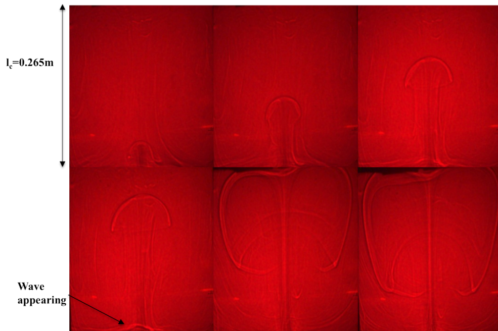
Figure 9.2: A wave seen developed in the conduit of the \Delta T=18^\circ\text{C} Golden syrup experiment.
