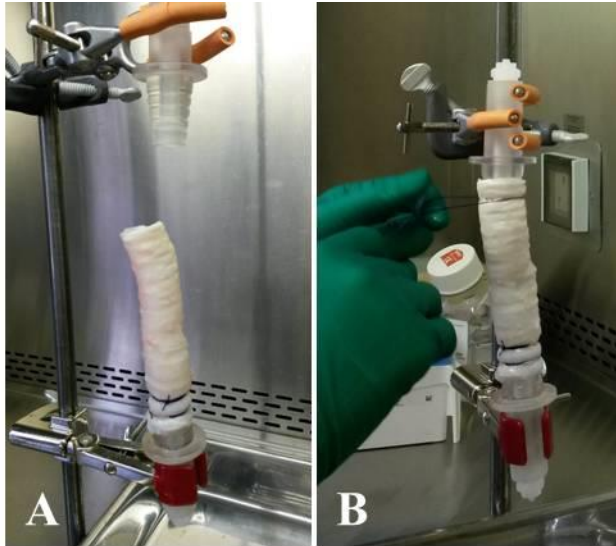
Figure 4.4: Attachment of the trachea to the SAC using sutures was aided by utilisation of a laboratory support stand (A) and clamps to hold the SAC and trachea in position (B).
