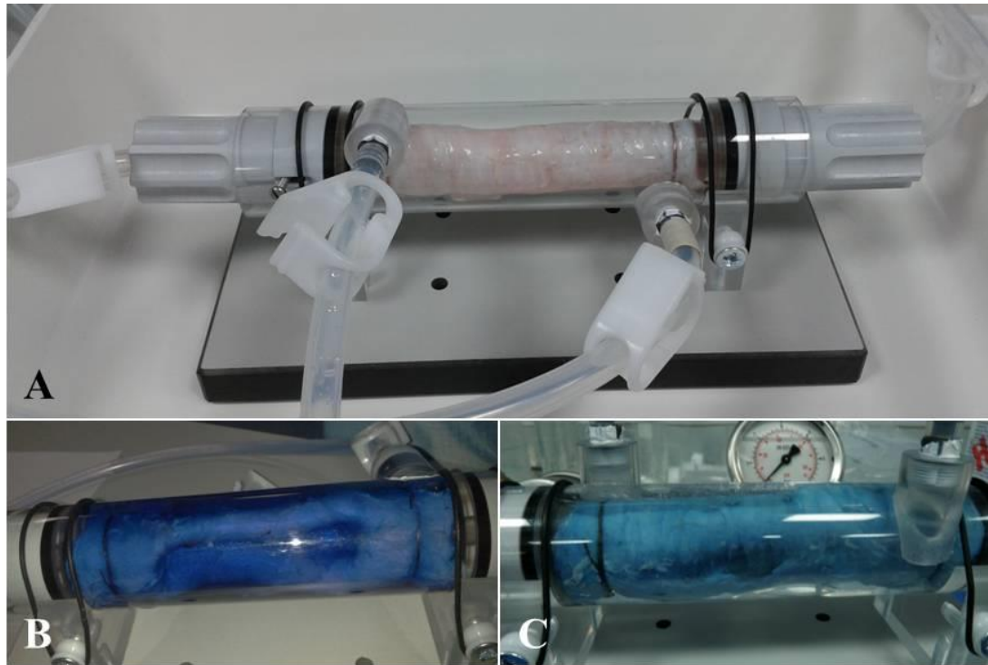
Figure 4.9: Stills from the initial transmural experiments demonstrate the trachea in position (A), the effect of external over-pressurisation (B) causing internal collapse of the trachealis muscle and the effect of internal over-pressurisation (C) causing external strain of the trachealis muscle.
