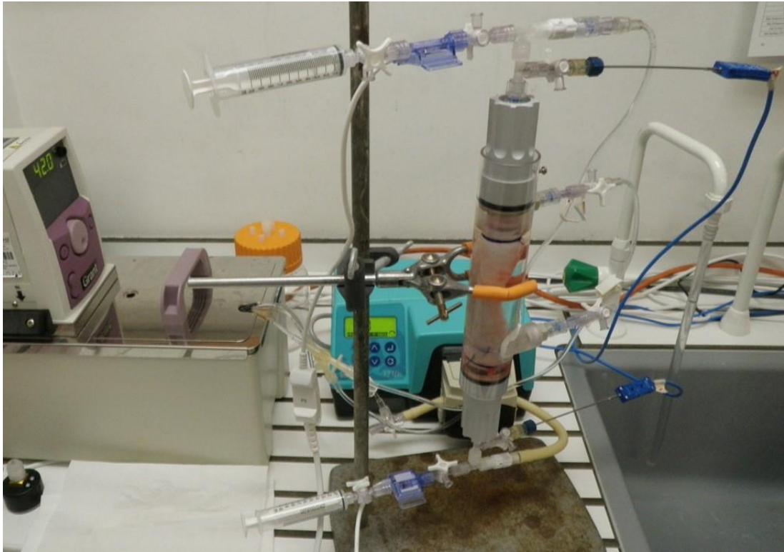
Figure 5.20: Bioreactor v2.3 which had extra ports included to allow for easy fill and drain of the decellularisation solutions.
