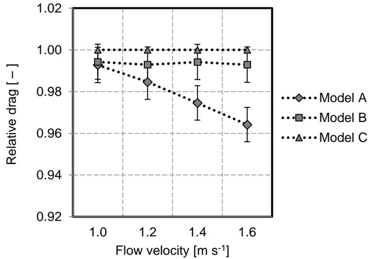
**Fig. 9. Relative drag for model trawls with 95% confidence intervals and model C being the benchmark [Model A: T0 body and T45 sides; Model B: T0 body and T0 side panels; Model C: T45 body and T0 sides].**
