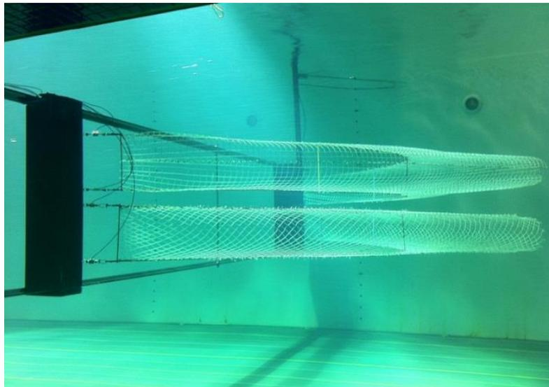
**Fig. 6. Two model trawls (A on top and B on bottom) attached to the Trawl Evaluation Rig in the middle section of the flume tank – T45 and T0 mesh in the wings can be noted in the upper and lower model respectively.**
