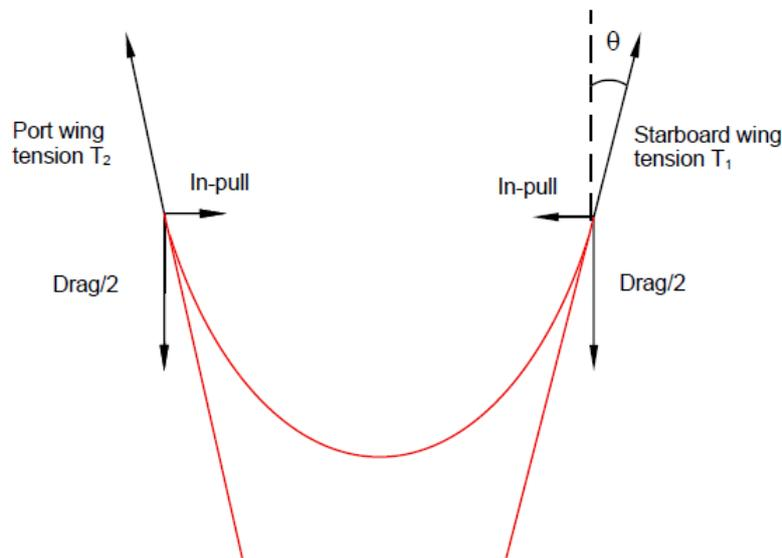
**Fig. 8. Force vector breakdown for a prawn trawl.**
