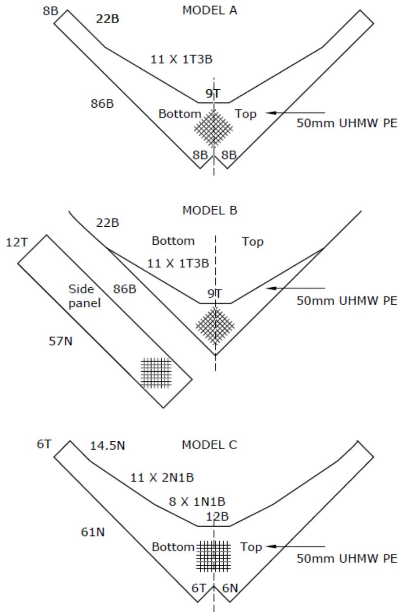
**Fig. 3. Net plans for Standard trawls: Model A [T0 body with T45 sides], Model B [T0 body with T0 sides], and Model C [T45 body with T0 sides]. N – normal, T – transversal, B – bar. Hanging ratio: E=0.71 for meshes on framelines and E=0.75 for side panel meshes to AB body taper of trawl B.**
