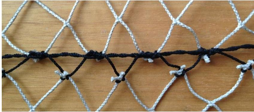
**Fig. 7. Bracing rope implementation along the longitudinal centre line of model MTA (hanging ratio  $E=0.71$ ).**
