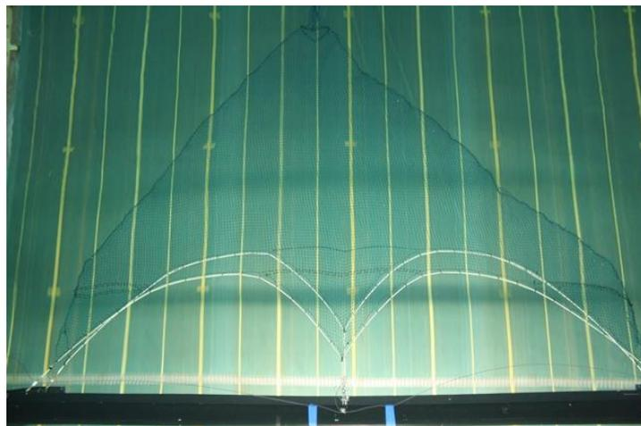
**Fig. 1. A model double-tongue trawl with netting hung square (T45) to the framelines, and built from knotted polyethylene – the model is asymmetric about the centre-line due to different mesh lengths down the port (T0) and starboard (T90) sides caused by differences in knot lengths in those two directions.**
