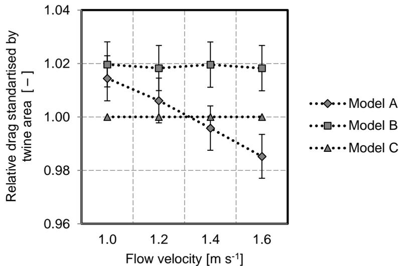
**Fig. 10. Relative drag standardised by twine area, with 95% confidence intervals and model C being the benchmark [Model A: T0 body and T45 sides; Model B: T0 body and T0 side panels; Model C: T45 body and T0 sides].**
