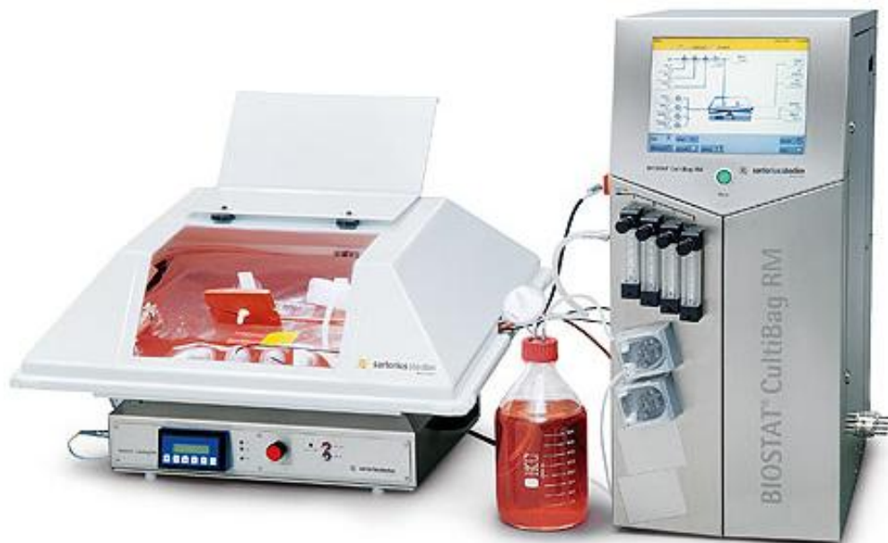
Figure 2.4: Sartorius BIOSTAT ® Cultibag RM rocking platform and control tower (image obtained from www.sartorius.co.uk , accessed 20.02.2014).
