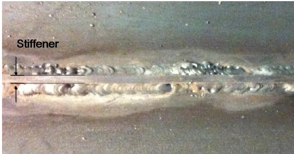
Fig 3.6 Large steel plate with welded stiffener of rectangular cross-section (5 mm thickness).
