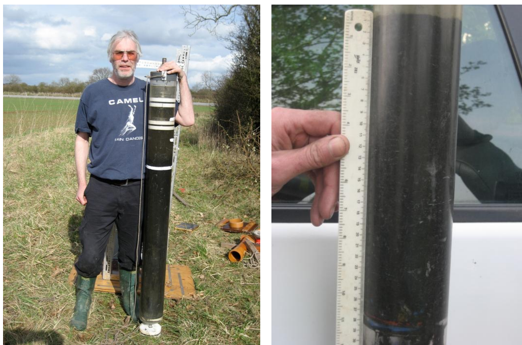
Figure 5.5. Left: Core RAIL1 collected from the Bodham Rail Pit using the ‘Big Ben’ piston corer in April 2010. Note the dark brown/black organic silt and lighter grey marl at the base of the core. Right: close-up of Core RAIL2 collected in August 2010 using a Glew gravity corer. (Photographs: Carl Sayer).
