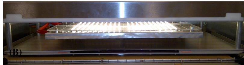
Figure II.8: Example images showing (A) set-up and utilisation of the SUPBr containing four days culture of C. sorokiniana . (B) a cross section of the suspended high power LED and the novel platform designed for the SUPBr. Light intensity in both cases were 180 \mu\text{mols.m}^{-2}.\text{s}^{-1} . Experiment performed as described in Section 2.3.2 & 2.5.3.
