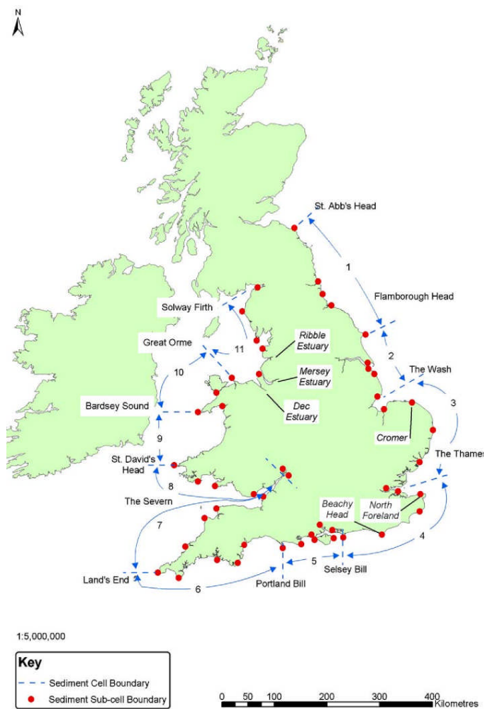
Figure 1.1 Sediment cells around the coast of England and Wales (adapted from Motyka and Brampton (1993), Cooper and Pontee (2006)).
