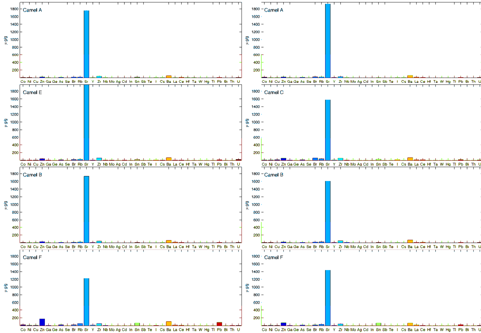
Figure 6.38 Minor/Trace element (XRF) composition (ug/g) of intertidal sediments at sampling sites in Camel Estuary.
