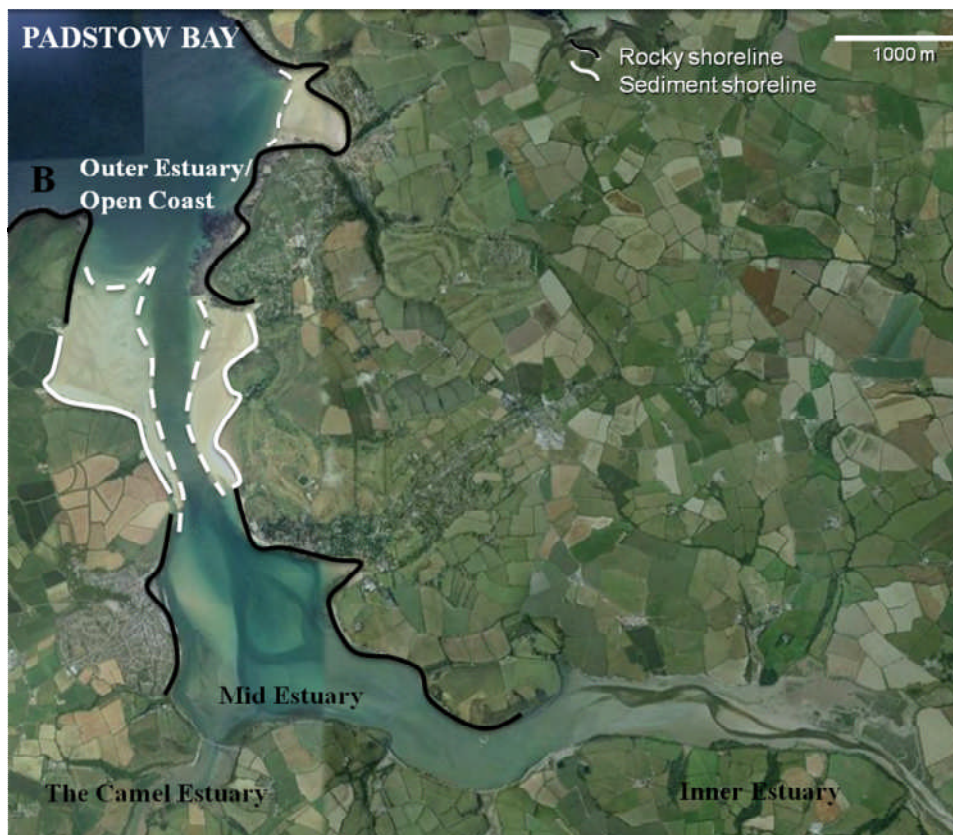
Figure 3.14 (A) The Padstow bay and Camel Estuary. Inset: Location in Southwest England, and (B) the the 20/08/2012 Google aerial photograph showing the sediment and rocky shoreline.
