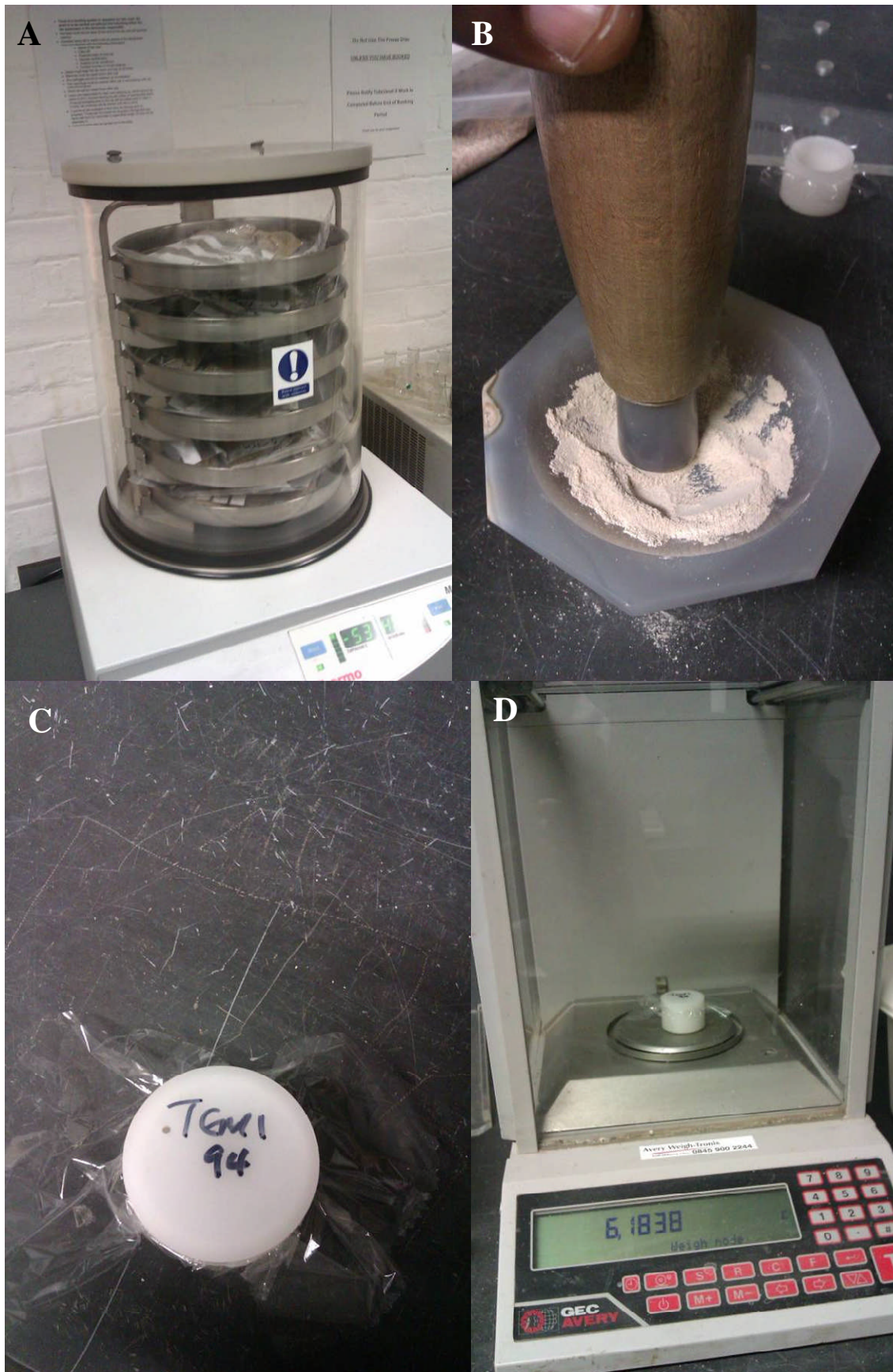
Figure 2.5 (A) MODULO 4k Freeze drier (B) pulverising into using agate mortar and pestle (C) storing the pulverised sample in compression die and (D) weighing the sample.
