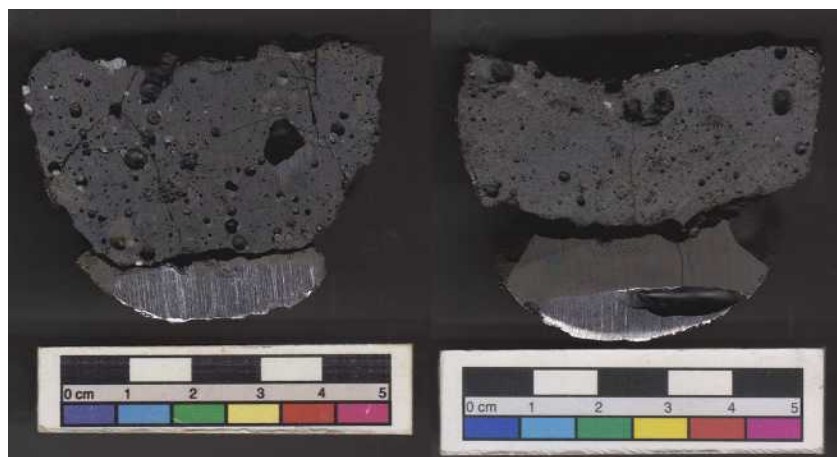
Fig. 15. Cross-sections of SL1 (left) and SL2 (right). The material inside the crucible separated into three layers. Top: slag, middle: matte, bottom: lead.
