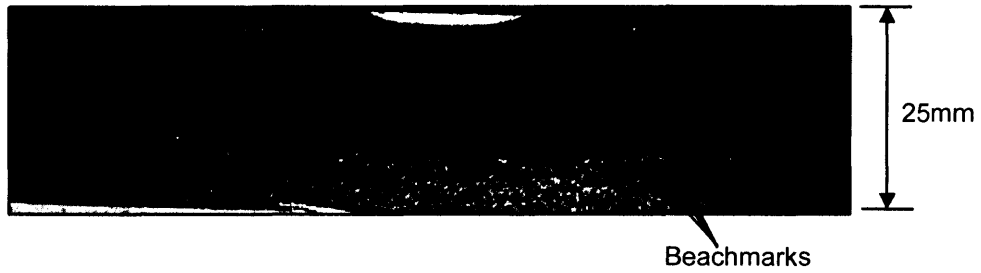
(a) Typical semi-elliptical surface crack grown under pure bending
