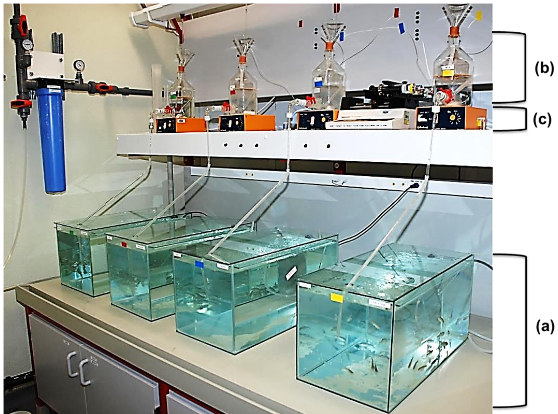
Figure 10. A continuous flow-through system used to expose fish to ibuprofen. Water flowed from an overhead trough into a 45 L glass tank (a) through a 2 L glass mixing vessel with an outlet (b). The mixing vessel was positioned on top of a magnetic stirrer (c) to ensure continuous mixing of test solutions before delivery into the respective tank. Water flowing through the tanks went to waste.
