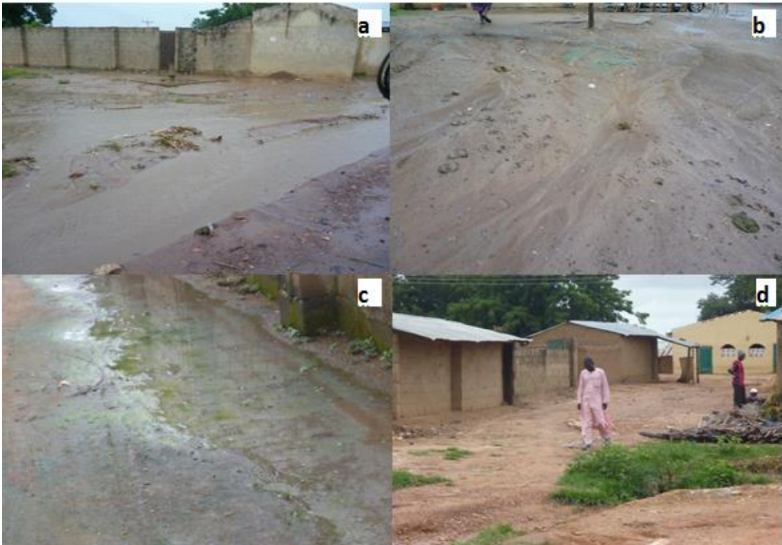
Figure 4.2: Illustrative surface conditions in the town landscape unit showing: a) runoff occurring a few minutes after the start of rainfall; b) evidence of sediment movement with runoff 30 minutes after the cessation of rainfall; c) retention of water within localised depressions one day after rainfall; and d) completely dry surface 3 days after rainfall
