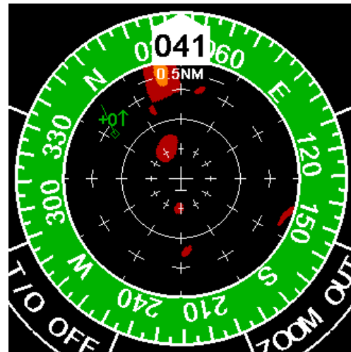
Figure 7.16: snapshot of the CDTI as soon as a terrain separation violation is detected
