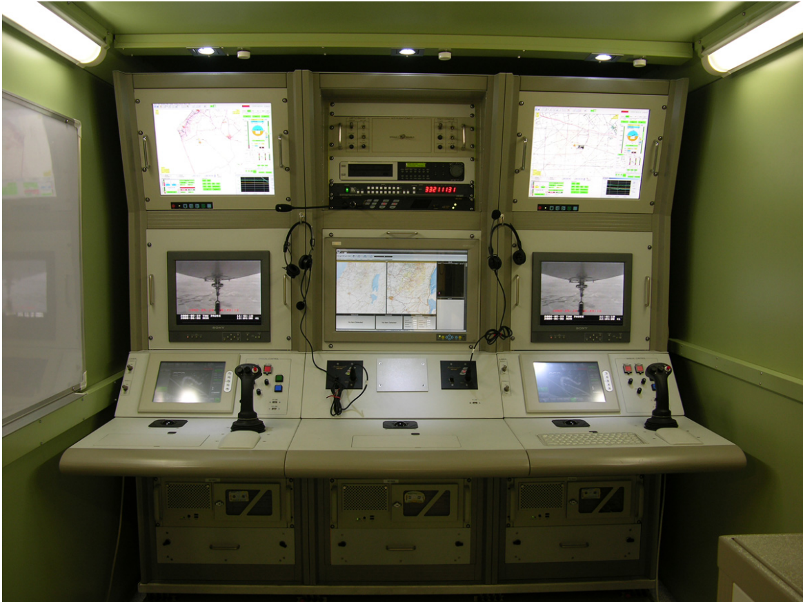
Figure 4.1: the GCS C4I System , a generic GCS for controlling various unmanned vehicle missions in real-time developed by Aeronautics . Source: [124]
