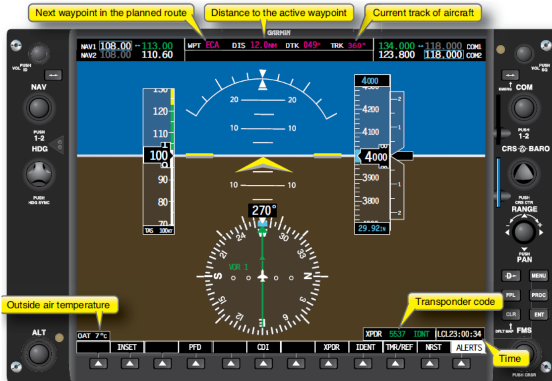
Figure 4.5: identification of the items used in PFD for communication of flight status information. Source: [125]
