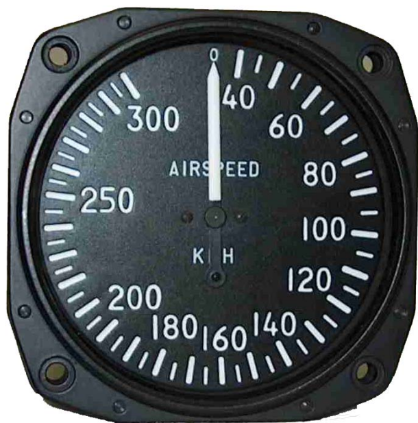
Figure 7.12: example of conventional steam gauge ASI [160]
