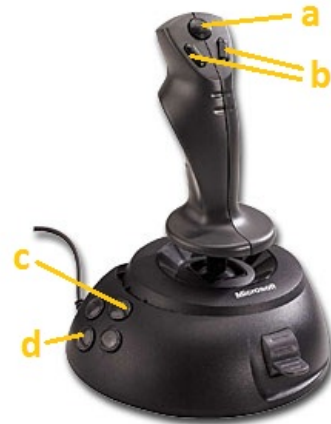
Figure 7.2: identification of the buttons functions on the Microsoft Sidewinder Joystick : a)elevator trim-up control, b)elevator trim-down control, c)rudder trim-right control, d)rudder trim-left control
