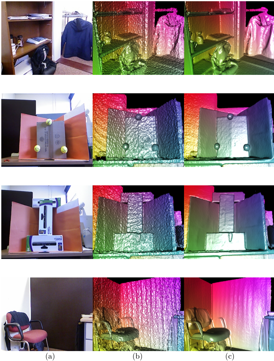
Figure 3.33 Experimental results for 3D on-line reconstruction applications. (a) RGB image. (b) 3D Scene reconstructed from raw depth data. (c) 3D Scene reconstructed from the filtered depth data
