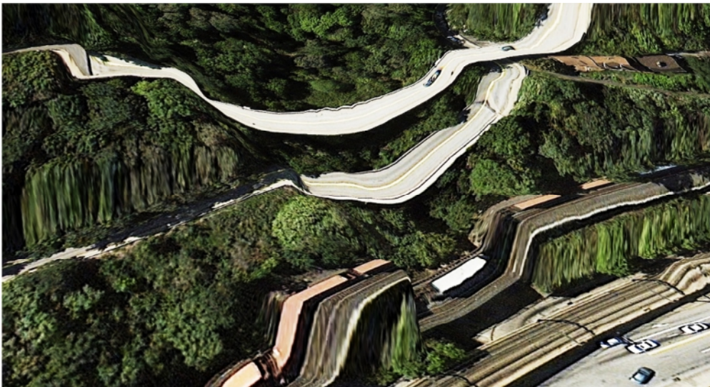
Figure 2.6 An example of an erratic mapping of texture on the 3D mesh of the terrain. Courtesy of Google Earth 6
