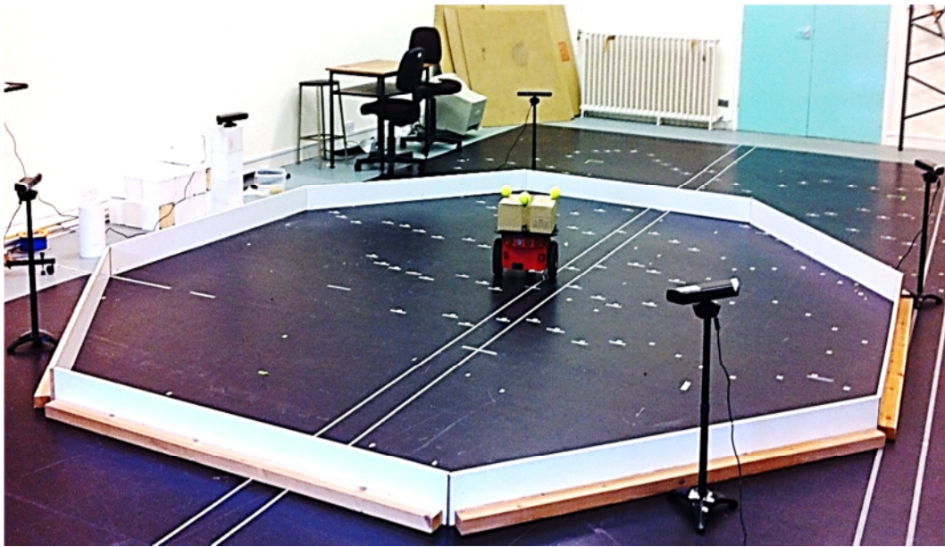
Figure 5.1 Multi-Kinect real-time tracking system
