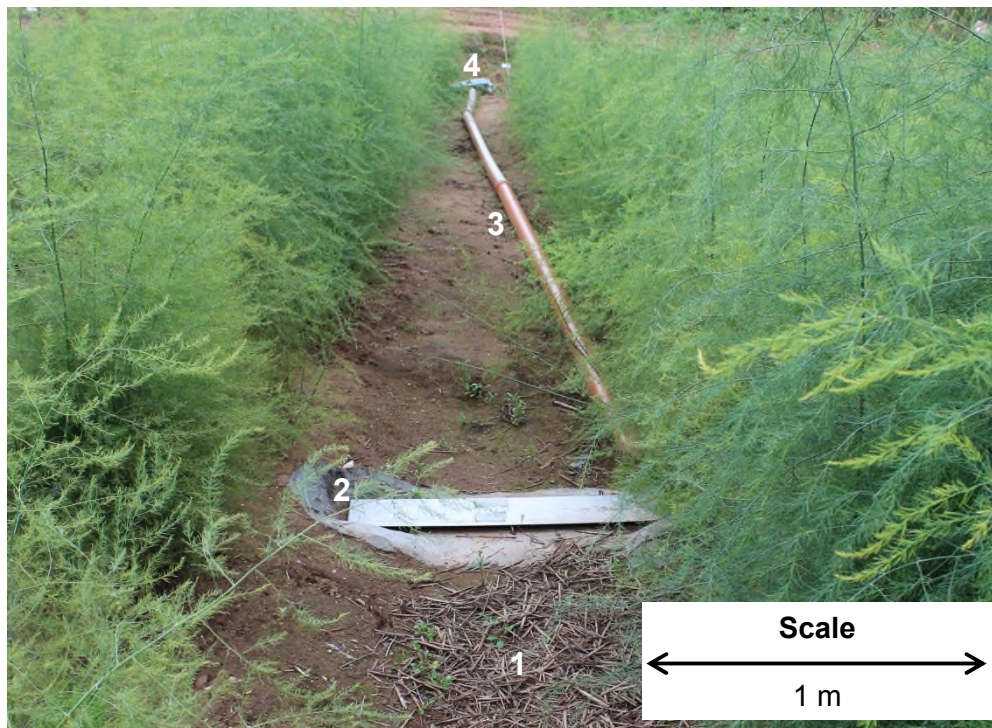
Figure 4.5. In-field experimental plot set-up (looking downslope from the treatment area). 1. Treatment area; 2. Gerlach trough; 3. Pipe; 4. Collection tank.
