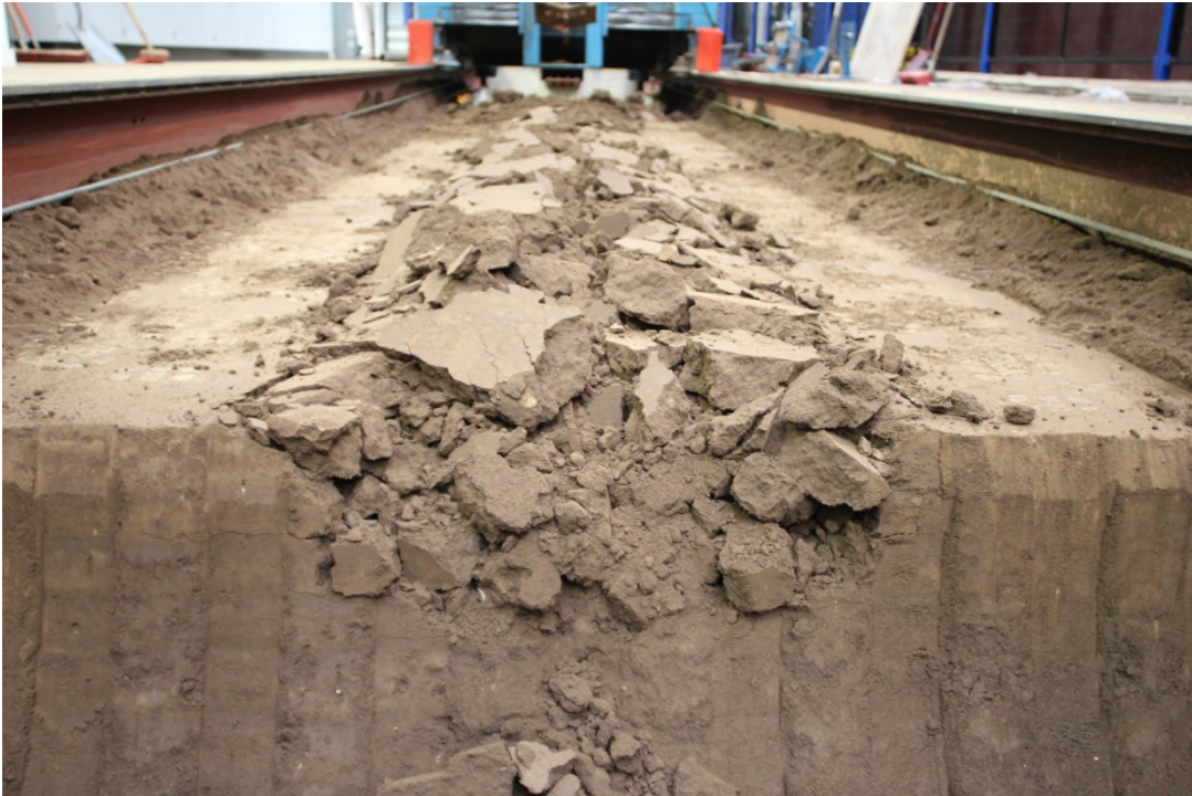
Figure_Apx B-12. Above ground disturbance at 300 mm resulting from the narrow tine (top image) and the winged tine (bottom image).
