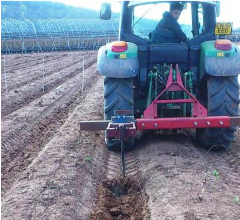
Figure 6.2. Shallow soil disturbance application using an offset mounted bracket.
