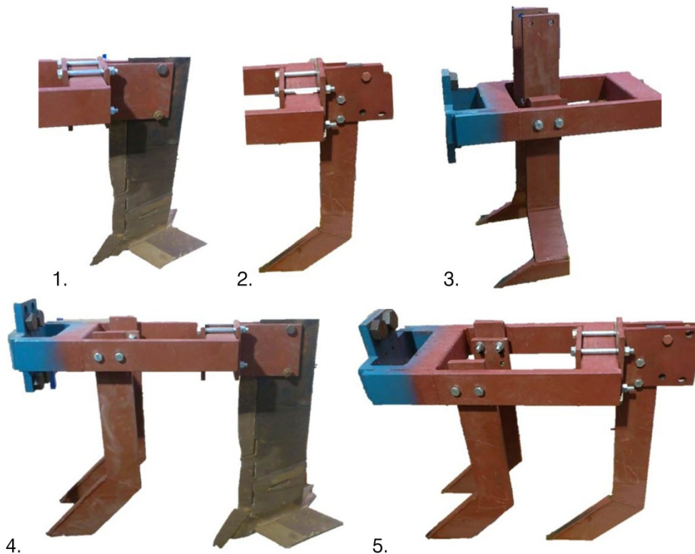
Figure 5.1. Tine configurations to be tested (not to scale); winged tine (WT; 1), narrow tine (NT; 2), modified para-plough (MPP; 3), winged tine with shallow
