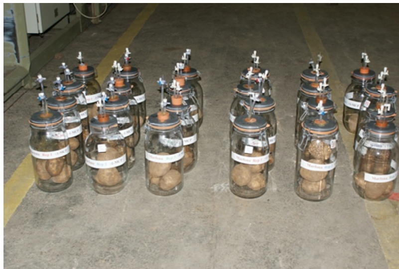
Figure 3.7 Three tubers per replicate were placed in 3L jars fitted with an air tight septum and gas measurements were taken
