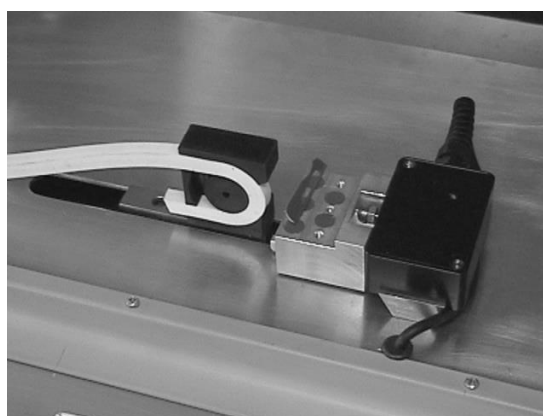
Figure 9. CATRA prototype sharpness measurement machine
