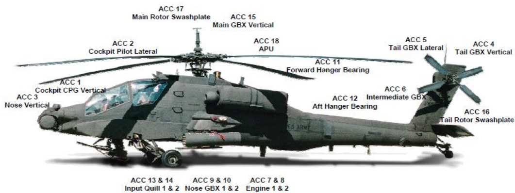
Figure 11 Accelerometer locations on AH64D HUMS
