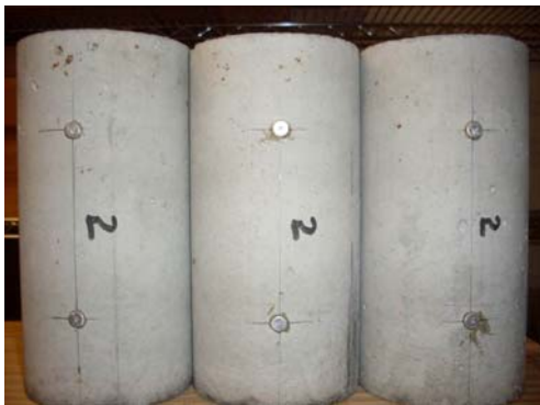
Figure 9. Concrete samples for laboratory tests.
