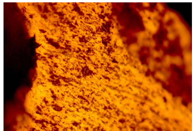
Fig. 8. Optical micrograph of a cell wall in a dolomite based foam produced with T_{\text{foam}} = 650\text{ }^{\circ}\text{C} , t_{\text{foam}} = 13\text{ min} , \rho^* = 0.705\text{ g/cm}^3 and \rho^*/\rho_s = 0.261 (50 \times ).
