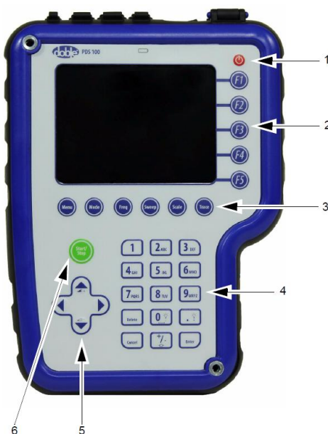
Fig. 4.3. Panel frontal del PDS-100 [32]
