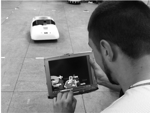
FIGURE 8 A sample picture of a user selecting the object of interest. It is indicated by the shape with a white border. The other objects are drawn with a different color.
