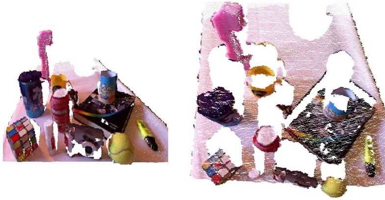
Fig. 2: Example of a point cloud from the Kinect camera. Left: view of the visible parts from everyday objects lying on a table. Right: same point cloud from top view, where empty gaps belong to occluded region and parts.
