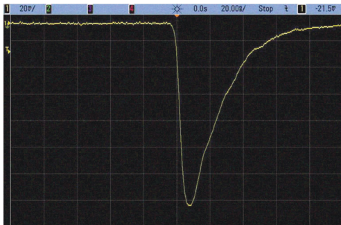
Figure 4: Anode signal of a 1'' \times 1'' \text{LaBr}_3(\text{Ce}) coupled to the R9779 Photomultiplier taken with a 2 Gs/s oscilloscope. The rise time of the signal from the 20% to maximum is 6 ns.
