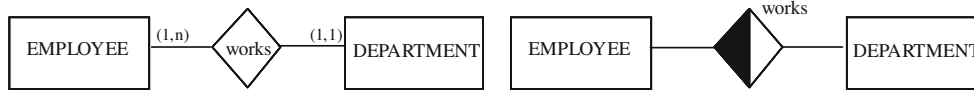
Fig. 1 Representing cardinality constraints in ECR model (left) and with Teorey notation (right)
