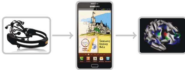
Figure 5.1: Main components of a mobile brain scanning system.
