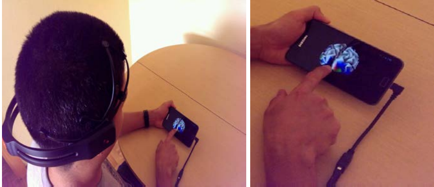
Figure 6.8: Online matrix factorization solver running on the Samsung Galaxy Note I (gray = no activity, blue = low activity, green = medium activity, red = high activity).
