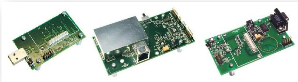
Figura 7: Gateway MIB520, MIB600 y MIB510, respectivamente
