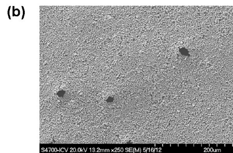
Figure 8. (a) XRD pattern of the HA + Y 2 O 3 sintered powder deposited on the Ti by EPD process and sintered at 1250 °C. (b) SEM micrograph of a general view of the surface of the sintered HA + Y 2 O 3 coating.
