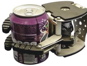
Figure 1.2: Fetch Hand grasping a can
