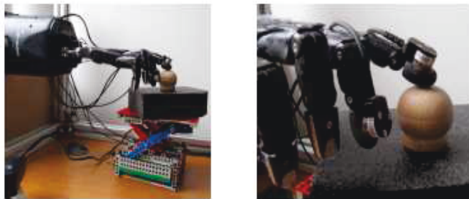
Figure 4.37: Shadow hand equipped by 6D force sensors at the fingertips
