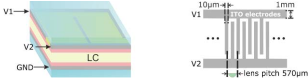
Fig. 1. Left: 3D view of the proposed scheme for a cylindrical LC lens. Right: Electrode pattern for the lens top plate. Note that, taking the right drawing as a reference, plates are located parallel to the paper plane. Sizes are not to scale.
