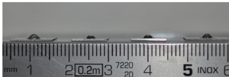
Figure 76. Small punch specimens of the Al-Mg-Si alloy after testing from left to right: CG condition, 1 ECAP passes and CR, 6 ECAP passes and CR and 4 ECAP-PP passes and artificially aged conditions.
