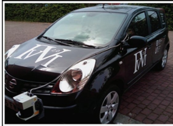
Fig. 1 Intelligent vehicle based on visual information (IVVI) 2.0
