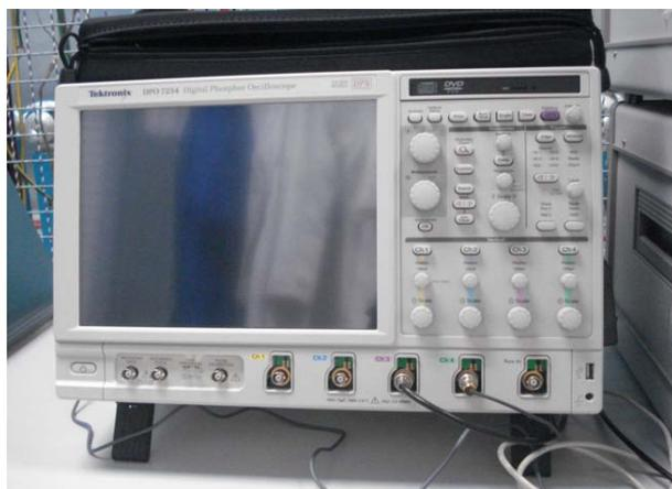
Figura B.4: Osciloscopio *Tektronix* DPO 7254.
