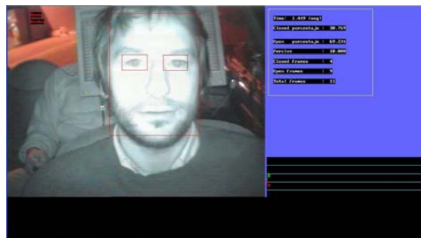
Figure 1.8: Somnolence monitoring as presented in [Flores et al. 2009]. Face and eyes are detected in both day and night configurations. The rate of blinking accumulated over time constitutes an indicator of somnolence on the driver.
