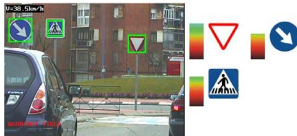
Figure 1.6: Traffic sign detection of [Carrasco et al. 2009]. Candidates are filtered by segmenting the image based on hue. A neural network is use to recognize the specific kind of traffic sign.
