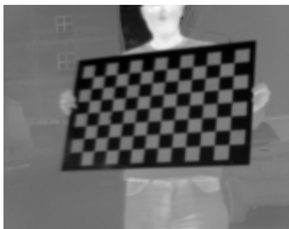
(a) Aluminum chessboard pattern in FIR.
