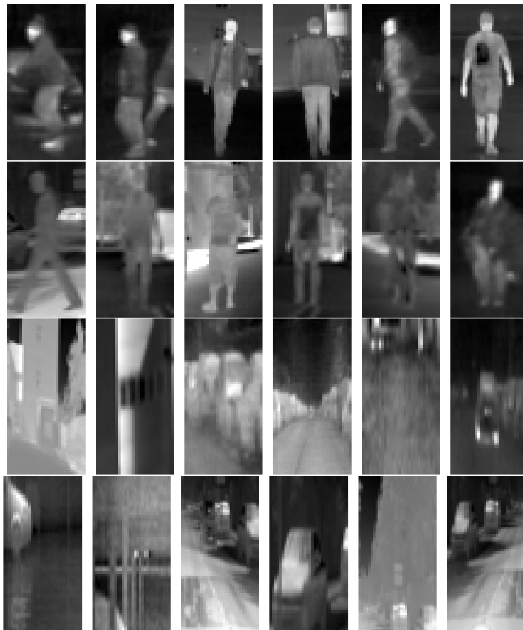
Figure 3.1: Example cropped-images of the classification dataset. The two upper rows contains examples of pedestrians acquired under different temperatures and illumination conditions. The lower rows contain randomly selected windows from images containing no pedestrians. For visualization purposes the contrast has been enhanced.
