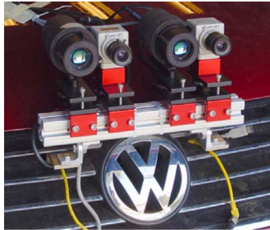
Figure 2.2: Tetracocular system used in [Krotosky and Trivedi, 2007a] made up of two VL and two FIR cameras.
